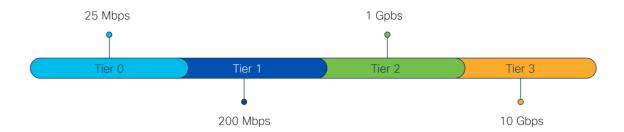
**Figure 7.**Four bandwidth tiers in Cisco DNA Software for SD-WAN and Routing
